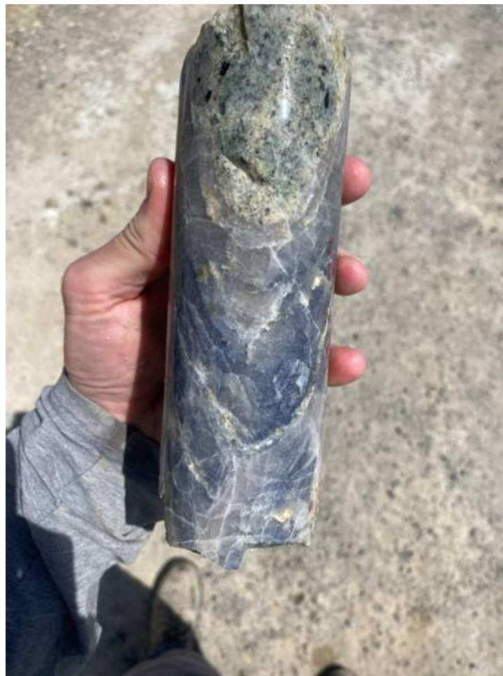
Figure 3: Quartz vein within potassic altered quartz-monzonite with very strong disseminated molybdenite (~10%) mineralisation throughout (Drillhole GCH-05 @ 123.8m).
