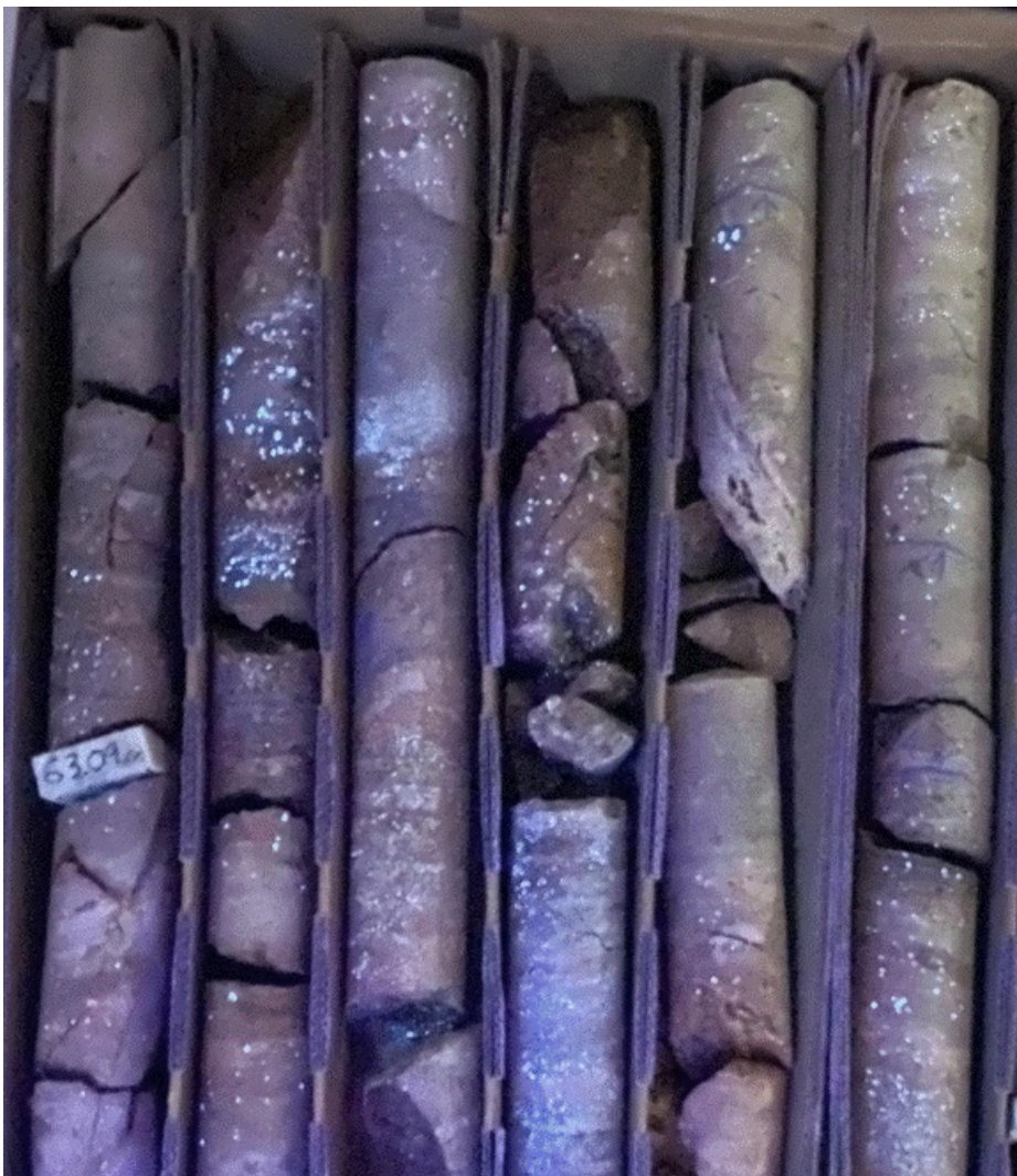
Figure 4: Pyrite and chalcopyrite mineralised quartz vein (Drillhole GCH-05 @ 136.8m).
