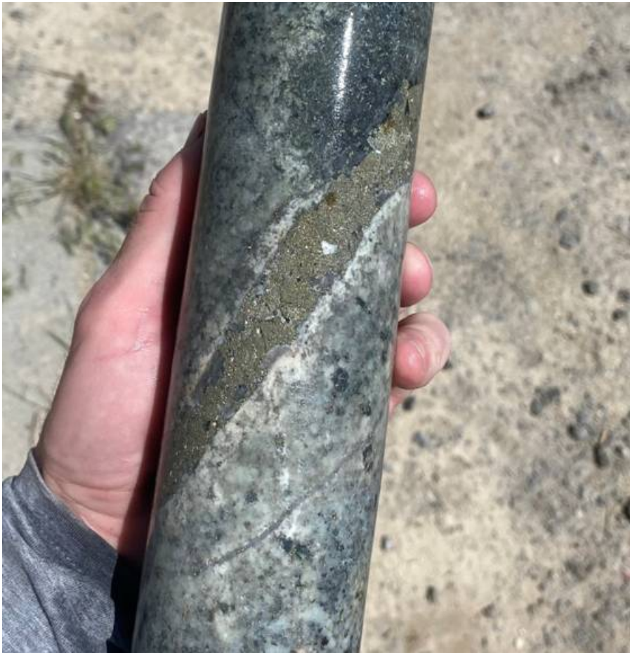
Figure 4: Pyrite and chalcopyrite mineralised quartz vein (Drillhole GCH-05 @ 136.8m).
