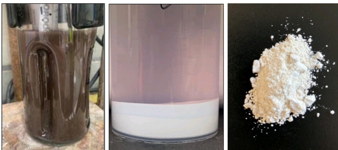
Figure 3. Purification and product finishing testwork, photos from left to right: titanyl sulphate solution from leaching stage, hydrated TiO 2 produced from hydrolysis, and the calcined TiO 2 product.
