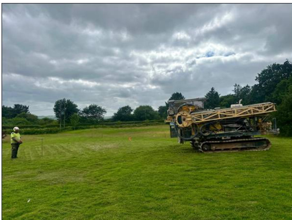
Figure 1: First diamond core drill rig on site at Redmoor, Cornwall
