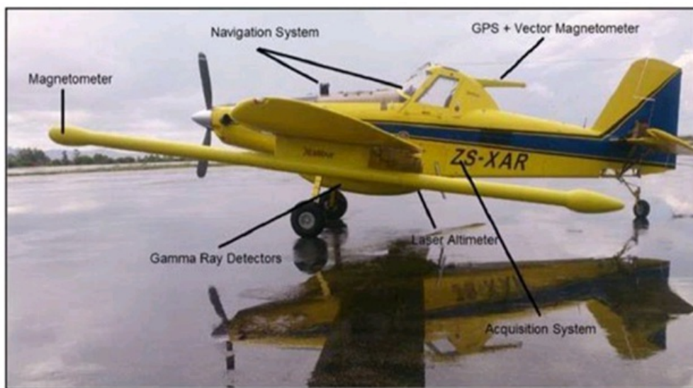
Image 2: Xcalibur 'air tractor' to be used for the gravity survey
