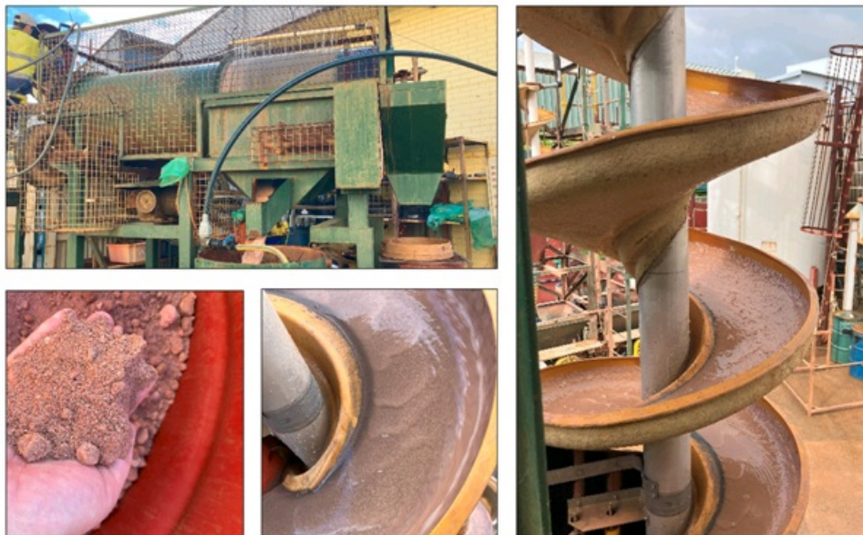
Figure 1. Photos of bulk testwork programme showing clockwise from bottom left: deslimed feed sample, wet scrubber unit, and gravity spirals .
