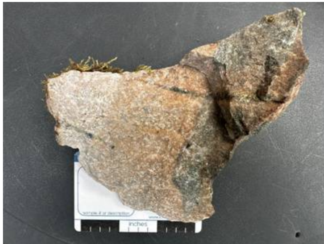
Figure 6 grab sample from the 'dump' near shaft B43 containing chalcopyrite (Cu mineral) and galena (Pb mineral)
