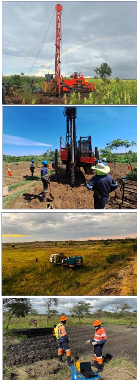
Figures 1-4 Clockwise from Top Left: Geotechnical diamond drilling, auger drilling, seismic geophysics testing using multi-channel analysis of surface waves (MASW), Cone Penetration Test with pore pressure measurements (CPTu) rig.
