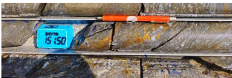
Figure 1. Significant visible copper mineralisation in drill core from MADD032, Mont Agoma prospect
