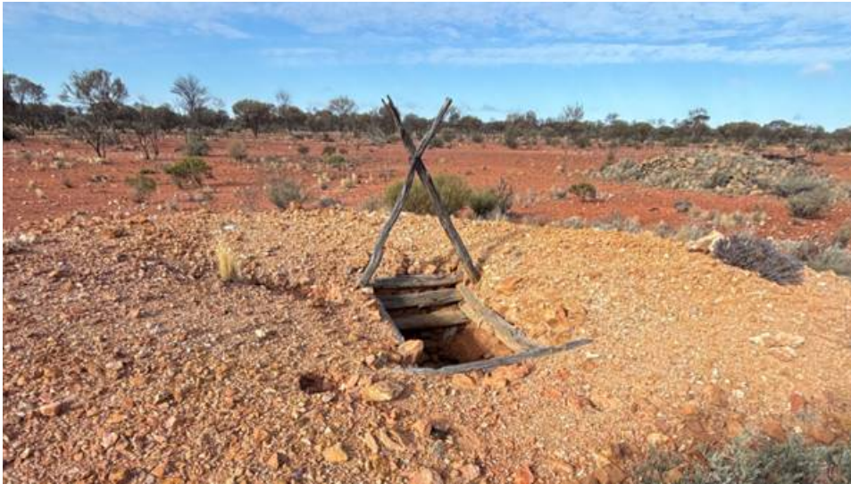
Figure 5: 15m Deep Shaft at Darlot West Project
