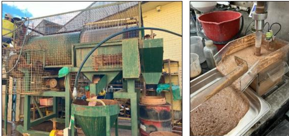
Figure 3. (L-R): Bulk Scrubber test in progress at AML, Batch slimes fraction rougher flotation test at ALS.
