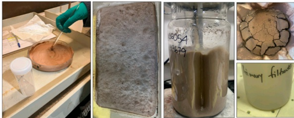
Figure 4. Elemental Extraction testwork (L-R): Acid-Concentrate mixing pre-acid bake, Acid bake product, initial stages of water leach, water leach residue and filtrate.
