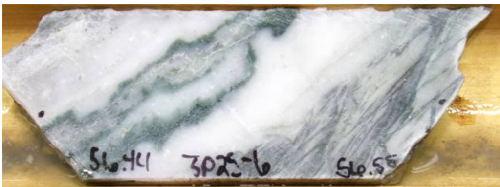
Figure 5 0.11m segment of half NQ core from Hole JP25-6 - 56.44m to 56.55m displaying a quartz-barite-sulphide vein near the Brown shaft of the Pioneer Mine Site on the Jennings Trend.
