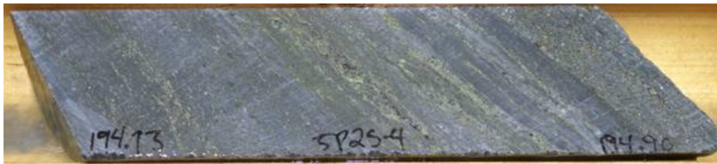
Figure 3 0.17m segment of half NQ core from Hole JP25-4 - 194.73m to 194.90m displaying foliation parallel sulphides found at the base of the Middle Zone of the Barite Hill Trend.
