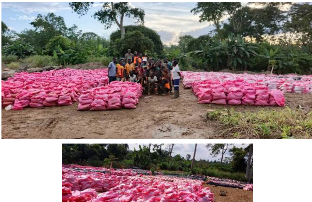
Figure 3: Bulk soil sample bags stored for each hole metre by metre, containing various quantities of heavy minerals and ready for processing using the pilot wash plant.
