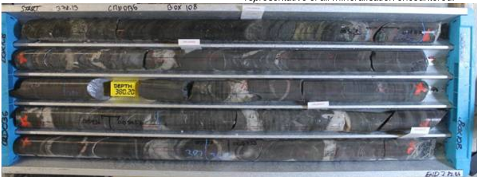
Figure 7: Example SVS-style mineralisation with quartz-greisen veins containing wolframite (tungsten) and minor chalcopyrite (copper) mineralisation in exploration drill core from drill hole CRD036. The core photograph shown is a selected example of logged drill core and is not necessarily representative of all mineralisation encountered. Core is to be sampled and laboratory assays will provide quantitative results.
