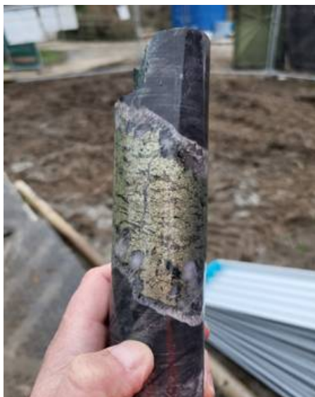
Figure 2: Example of chalcopyrite (copper) and minor cassiterite (tin) mineralised exploration drill core from
