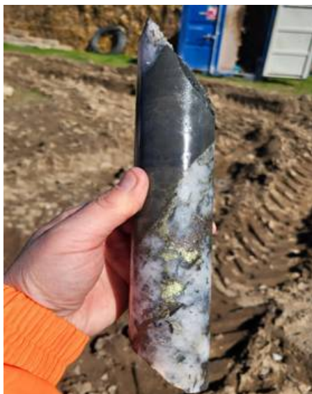
Figure 1: Example of coarse wolframite (tungsten) minerals and chalcopyrite (copper) mineralised
