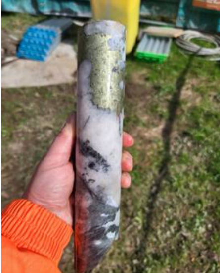
Figure 3: Example of coarse wolframite (tungsten) minerals and chalcopyrite (copper) mineralised exploration drill core from drill hole CRD037. The core photograph shown is a selected example of logged drill core and is not necessarily representative of all mineralisation encountered.
