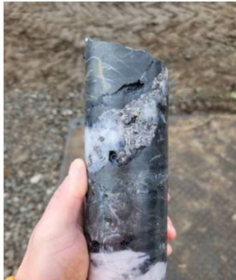
Figure 6: Example of lode-style mineralisation with quartz veins containing cassiterite (tin) and minor chalcopyrite (copper) mineralisation in exploration drill core from drill hole CRD039, outside of the Redmoor SVS. The core photograph shown is a selected example of logged drill core and is not necessarily representative of all mineralisation encountered.
