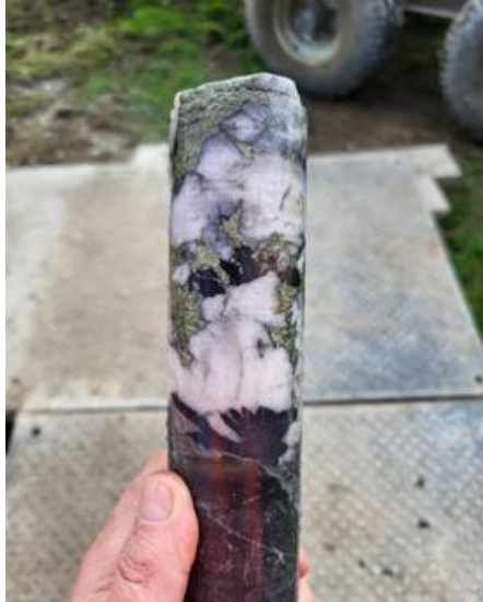
Figure 4: Example of coarse wolframite (tungsten) minerals and chalcopyrite (copper) mineralised exploration drill core from drill hole CRD037. The core photograph shown is a selected example of logged drill core and is not necessarily representative of all mineralisation encountered.
