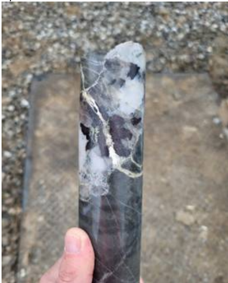
Figure 5: Example of coarse wolframite (tungsten) minerals and minor chalcopyrite (copper) mineralised exploration drill core from drill hole CRD038. The core photograph shown is a selected example of logged drill core and is not necessarily representative of all mineralisation encountered.
