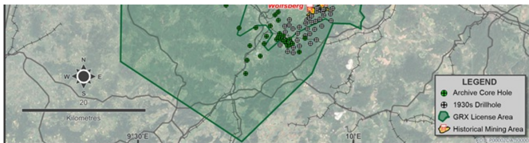
Figure 4: Location Map of GreenX's Tannenberg project area showing the newly discovered 95 x 1930s drillholes, the location of the three underground copper/ silver mines opened during the late 1930s, and the location of the modern era 47 archive core holes that GreenX now has access to for re-logging and sampling
