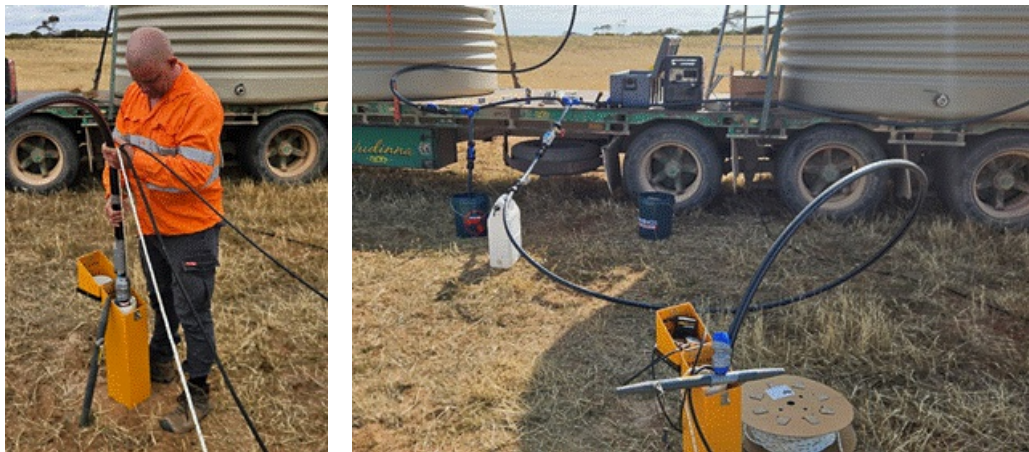
Figure 1. Rendement Principal Hydrologist Ben Jeuken installing a downhole pump in the Boland Wellfield and the pump test currently underway.
