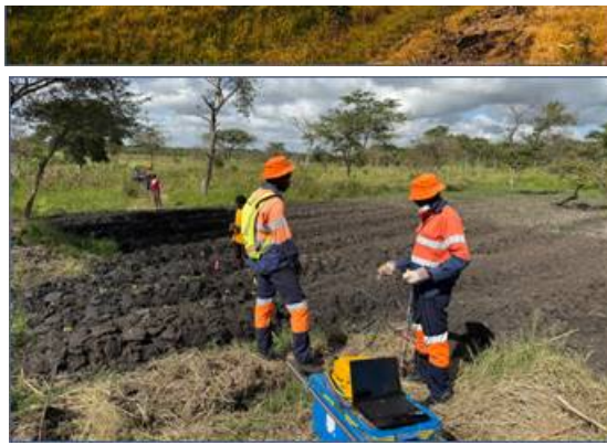
Figures 3-6 Clockwise from Top Left: Geotechnical diamond drilling, auger drilling, seismic geophysics testing using multi-channel analysis of surface waves (MASW), Cone Penetration Test with pore pressure measurements (CPTu) rig.
