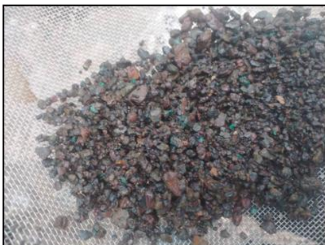
Figure 3. Field sample from drill hole 25TMNRC-043 showing visible secondary copper mineralisation (the green mineral, predominantly malachite).
