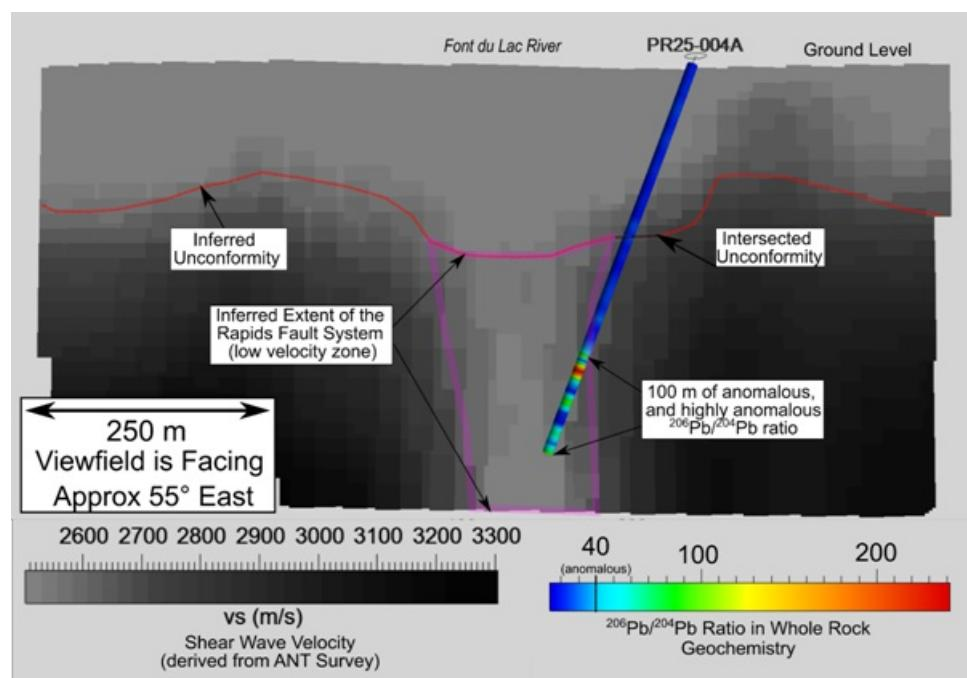
Notes: Downhole location of the highly anomalous  $^{206}\text{Pb}/^{204}\text{Pb}$  results in hole PR25\_04A overlain on a cut section (facing 55° East) of Ambient Noise Tomography survey data. Note the location of the highly anomalous  $^{206}\text{Pb}/^{204}\text{Pb}$  results within the inferred extent of the Rapids Fault System.
