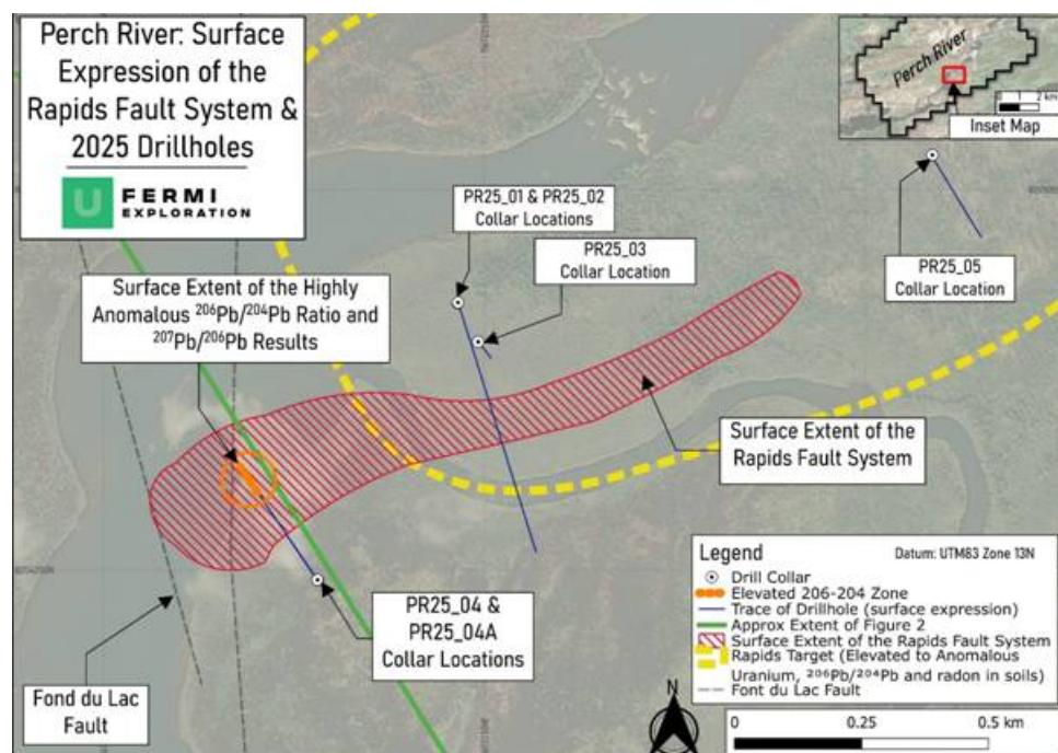
Notes: Drill collars & trace of the 2025 drilling shown with the location of the highly anomalous  $^{206}\text{Pb}/^{204}\text{Pb}$  and  $^{207}\text{Pb}/^{206}\text{Pb}$  ratio results. Major local faulting, and the extent of the Rapids Zone, an area of highly anomalous geochemistry in soils determined through fieldwork in 2024 is also marked.
