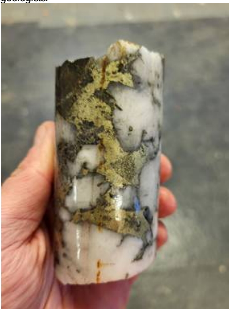
Figure 5: Example of chalcopryite (copper) in mineralised exploration drill core from drill hole CRD041, as logged & sampled by CRL geologists.
