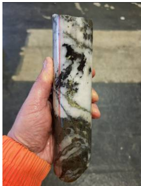
Figure 3: Example of very coarse wolframite (tungsten) and chalcopryite (copper) in drill core from drill hole CRD041, as logged & sampled by CRL geologists.
