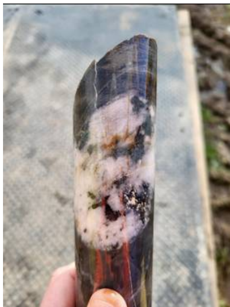
Figure 4: Example of coarse wolframite (tungsten) minerals in mineralised exploration drill core from drill hole CRD041, as logged & sampled by CRL geologists.
