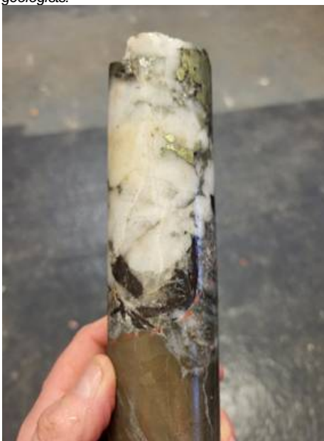
Figure 6: Example of coarse wolframite (tungsten), cassiterite (tin) and chalcopryite (copper) in mineralised exploration drill core from drill hole CRD041, as logged & sampled by CRL geologists.
