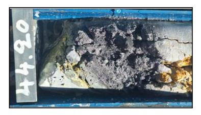
A narrow, but strongly mineralised massive sulphide vein encountered early in hole HMO-010, at 44.20m depth. The target to the main lode of mineralisation is 250m below the surface. Drilling continues, with this hole already at 75.60m depth in better ground conditions.
