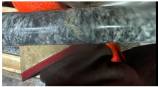
Figure 2 showing a section of uncut core from the Dead Otter trend displaying sulphides which could indicate potential mineralisation.
