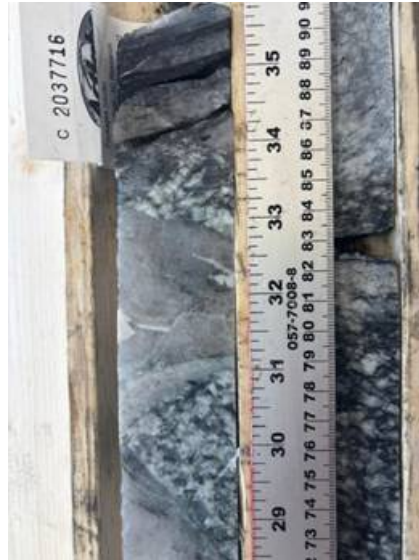
Figure 3 showing cut core displaying quartz veining and coarse pyrite.
