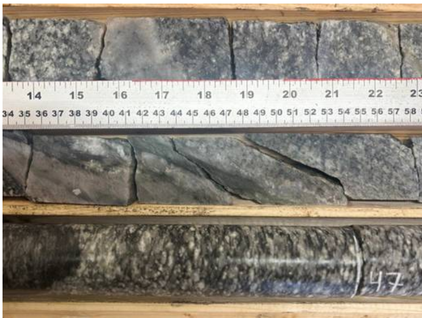
Figure 5 showing silicified, fractured granodiorite with shearing and quartz veins (with chlorite/ mylonite?) occupying the shear planes
