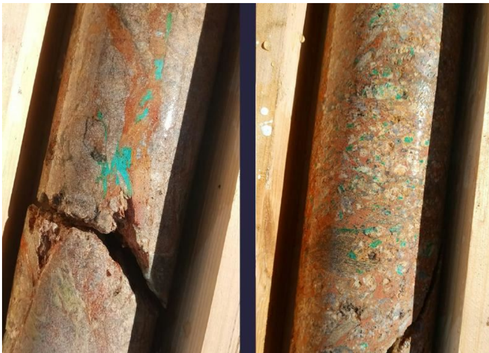
Â Fig.1 First drill core from recently commissioned diamond drilling rig with observable copper mineralisation
