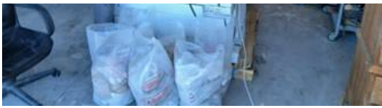
Above: Boxed core samples from sonic drilling in storage. Samples being tested for moisture content. Sepiolite, due to its high absorbency can contain as much as 50% moisture.
