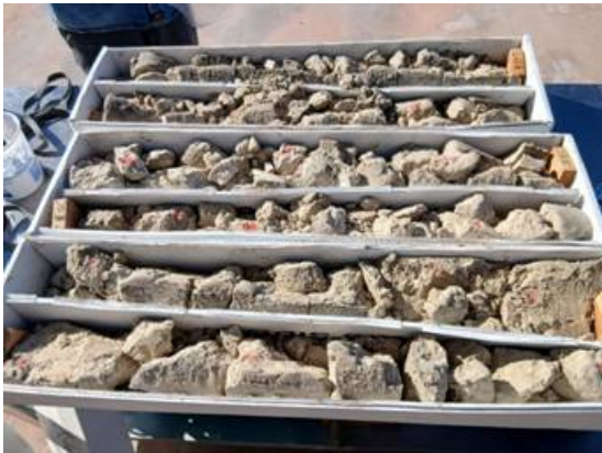
Above: Boxed core samples from sonic drilling in storage. Samples being tested for moisture content. Sepiolite, due to its high absorbency can contain as much as 50% moisture.
