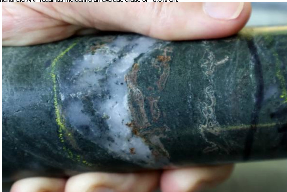
Figure 1: Drill core showing visible cassiterite (brown) within a broader ~2.0 m mineralised interval, with portable handheld XRF readings indicating an average grade of ~8.3% Sn.
