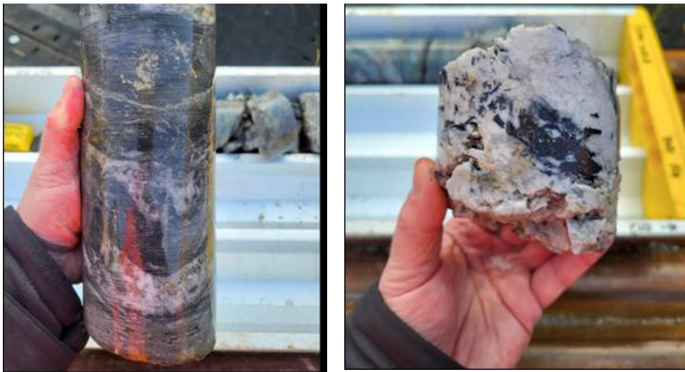
Figure 2: Chalcopyrite (left) and Wolframite (right) mineralisation within drillcore, visually logged by CRL Exploration Geologists between 32-34m depth downhole in CRD042.
