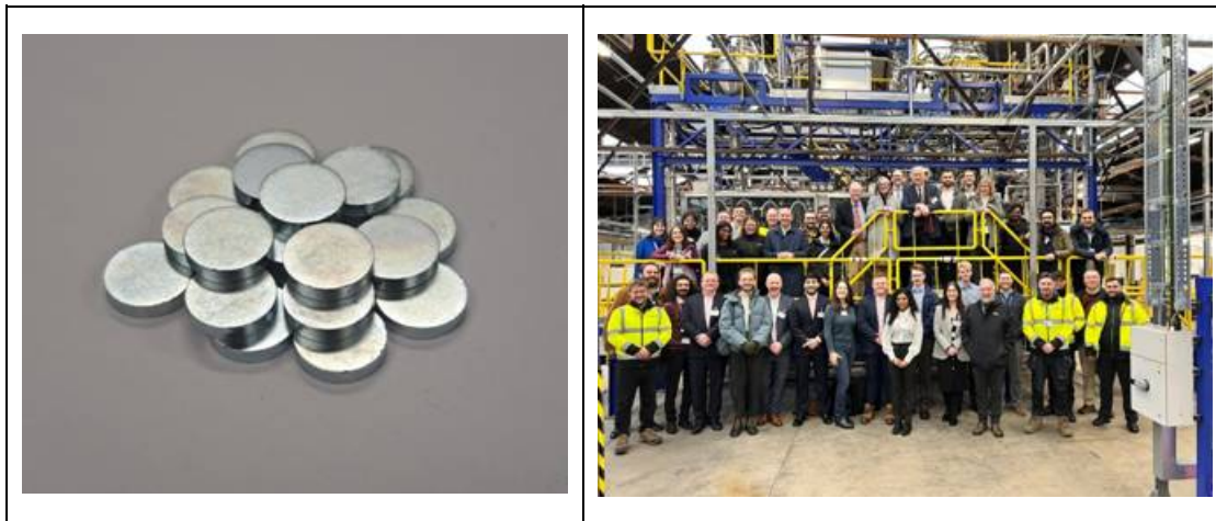
Left: Finished coated recycled NdFeB magnets for prototype demonstrations in medical devices.
