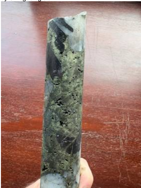
Figure 3: Example of massive chalcopyrite (copper) and very coarse wolframite (tungsten) in drill core from drillhole CRD042, as logged & sampled by CRL geologists.
