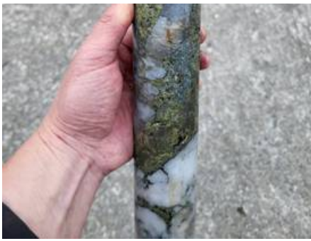
Figure 1: Example of very coarse wolframite (tungsten) and massive chalcopyrite (copper) in drill core from drillhole CRD042, as logged & sampled by CRL geologists.
