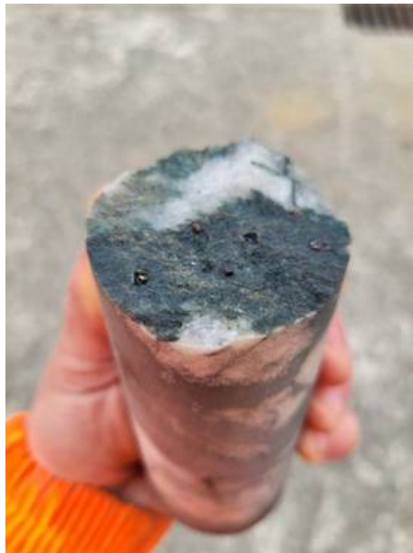
Figure 4: Example of coarse cassiterite (tin) minerals in mineralised exploration drill core from drillhole CRD042, as logged & sampled by CRL geologists.
