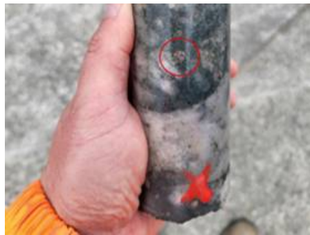
Figure 2: Example of fine cassiterite (tin) in drill core (e.g. red circle) from drillhole CRD042, as logged & sampled by CRL geologists.
