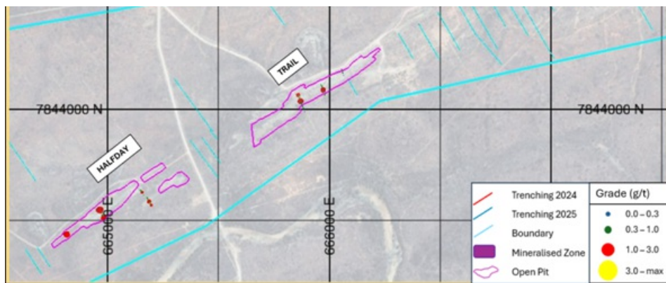
Figure 9: Plan view of Motapa South showing grade (g/t) intersections
