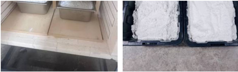
Fig. 2: Lithium Carbonate in drying kiln and product in bulk storage (Empower)
