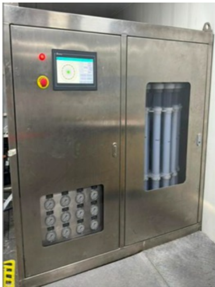
Fig. 3: LiCl Adsorption-Adsorbent Washing-Desorption Module (Lanshen)
