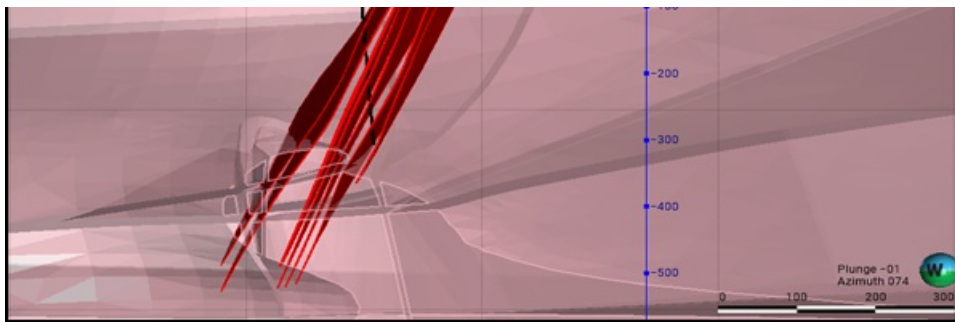
Figure 3: Cross-sectional view of drillhole trace for CRD044_D1, showing its relationship to high-grade domains (red for tungsten) intersected by CRD044_D1 with granite body (pink) as background.
