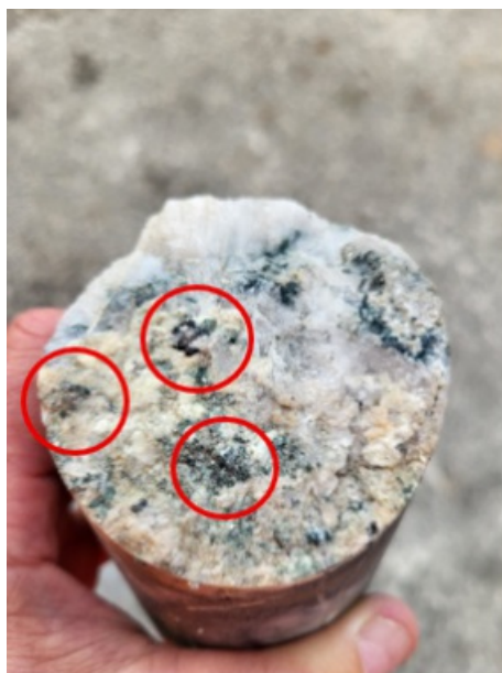
Figure 4: Example of coarse cassiterite (tin) minerals in mineralised exploration drill core from drillhole CRD049, as logged & sampled by CRL geologists.
