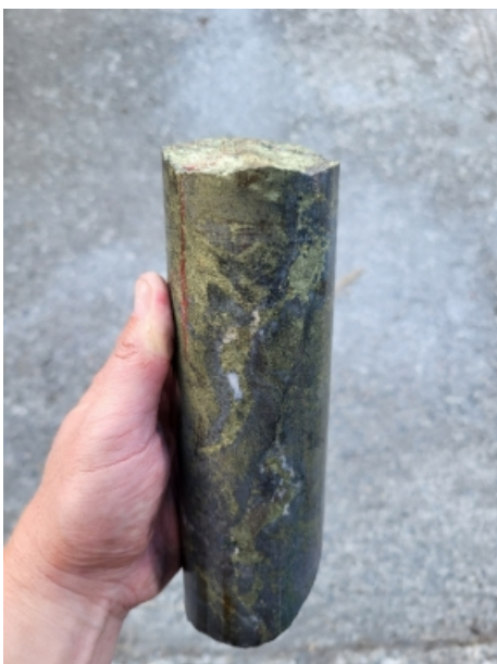
Figure 3: Example of massive chalcopyrite (copper) and very coarse wolframite (tungsten) in drill core from drillhole CRD048, as logged & sampled by CRL geologists.
