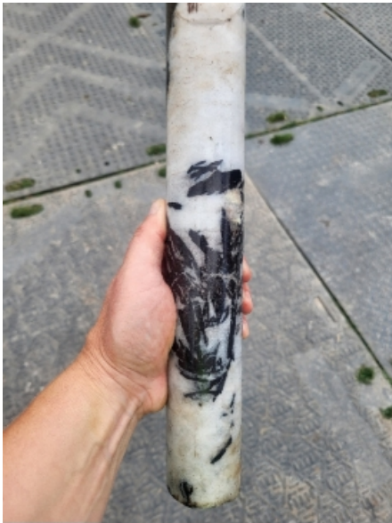
Figure 1: Example of very coarse wolframite (tungsten) in drill core from drillhole CRD047 as logged & sampled by CRL geologists.
