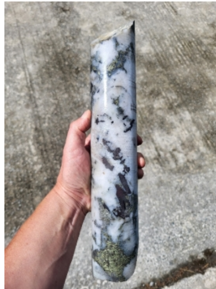
Figure 2: Example of coarse wolframite (tungsten) and chalcopyrite (copper) in drill core from drillhole CRD045, as logged & sampled by CRL geologists.
