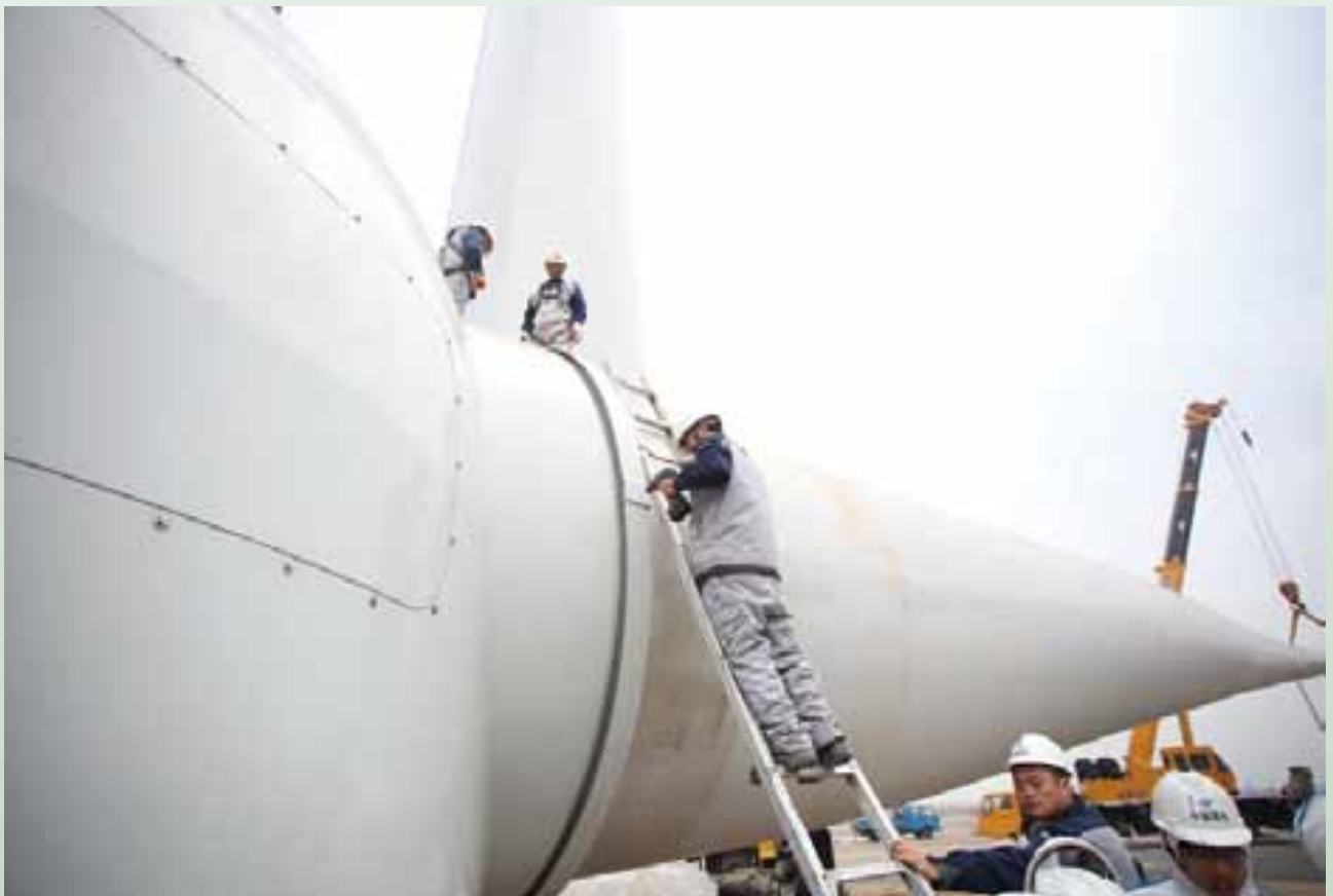
The generator of the 6MW double-fed offshore WTG 6MW海上雙饋風電機組發電機
