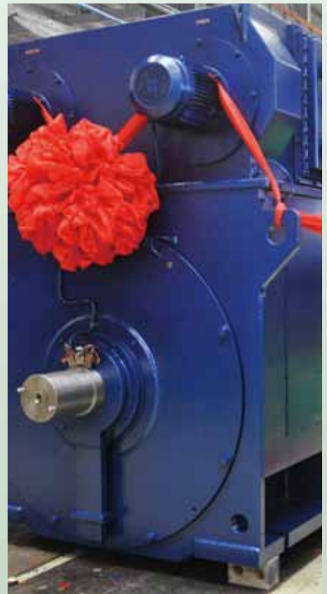
The generator of the 6MW double-fed offshore WTG 6MW海上雙饋風電機組發電機
