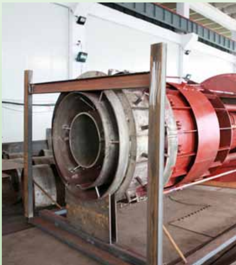
The first batch of low-NOx swirl chamber produced in 2012 2012年首批低氮旋流燃燒器
