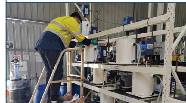
Carbonate product precipitation circuit setup
