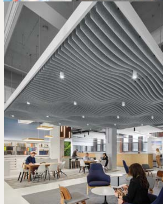
Middle: Optima® Tegular Ceiling Panels with Suprafine® XL® 9/16" Exposed Tee System
