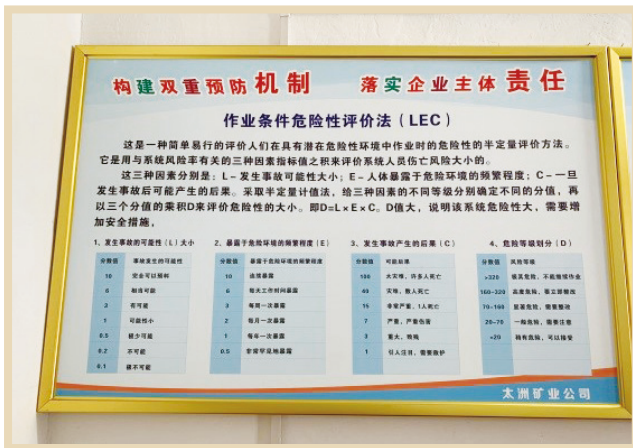
Method of Risk Assessment for Operation Conditions in Mines 於礦山的作業條件危險評價辦法
