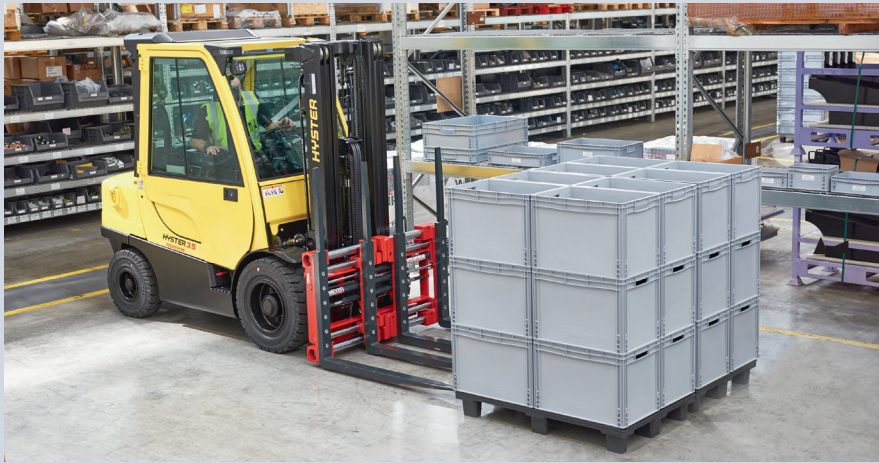
▲ The Veracitor® VX series lift truck is designed for medium- to heavy-duty applications. Here a GC050VX is equipped with a Bolzoni bale clamp.
