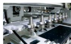
ND712DL 配置 2 组 8 刀位自动换刀刀库 2 sets 8-slot tool magazine of NCB612DPTL
