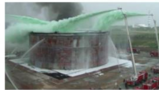
Three Triple-phase towers attacking full surface fuel fire (Source: Mingguang Hanhao Valhalla) 明光浩淼
