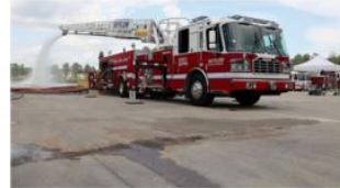
The Ferrara Skyflow producing 18,000 l/min at the tip (Source: Pinterest).
