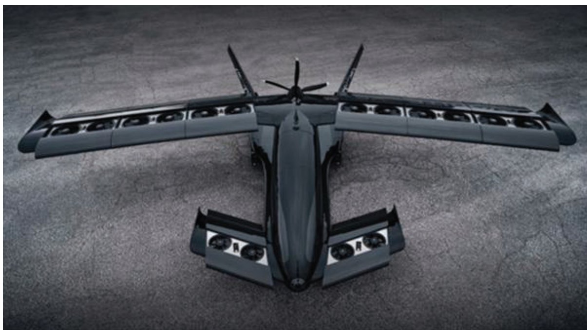
A picture of Horizon’s 50%-scale prototype that is currently in active flight testing
