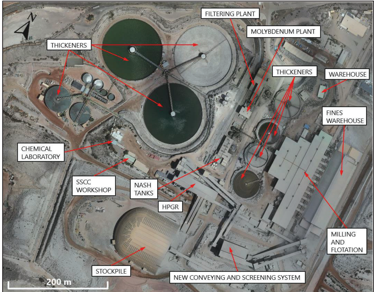
Figure 15-2: Process Plant Site Infrastructure
