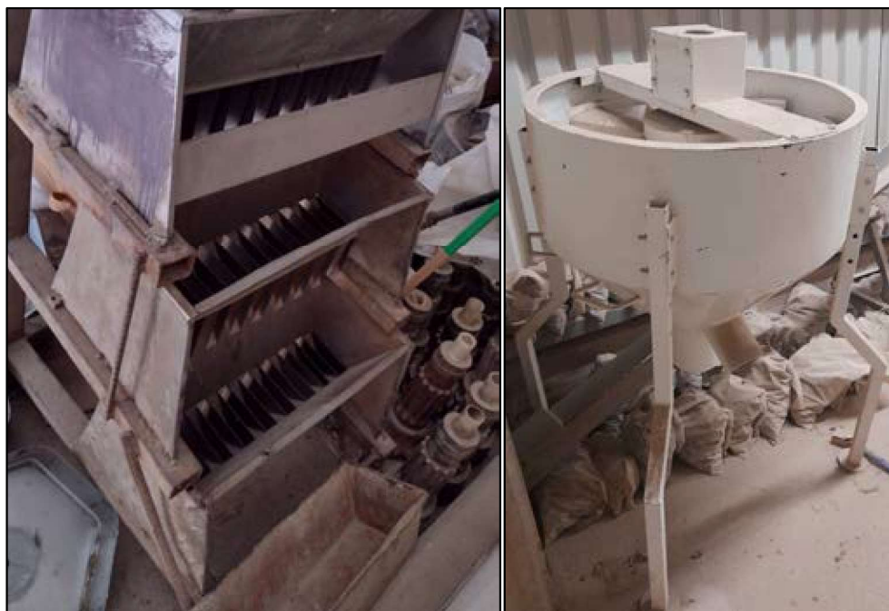
Figure 8.1: Jones Splitter – RC Sample Splitter, Left, Mechanical Splitter, Right
