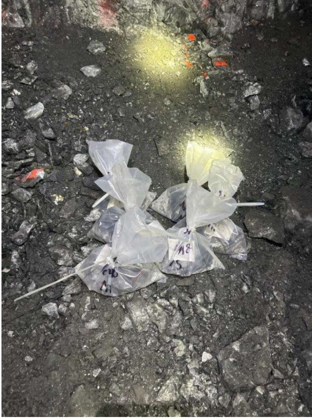
Figure 7-4: Sampling Collected and Sealed after Sampling
