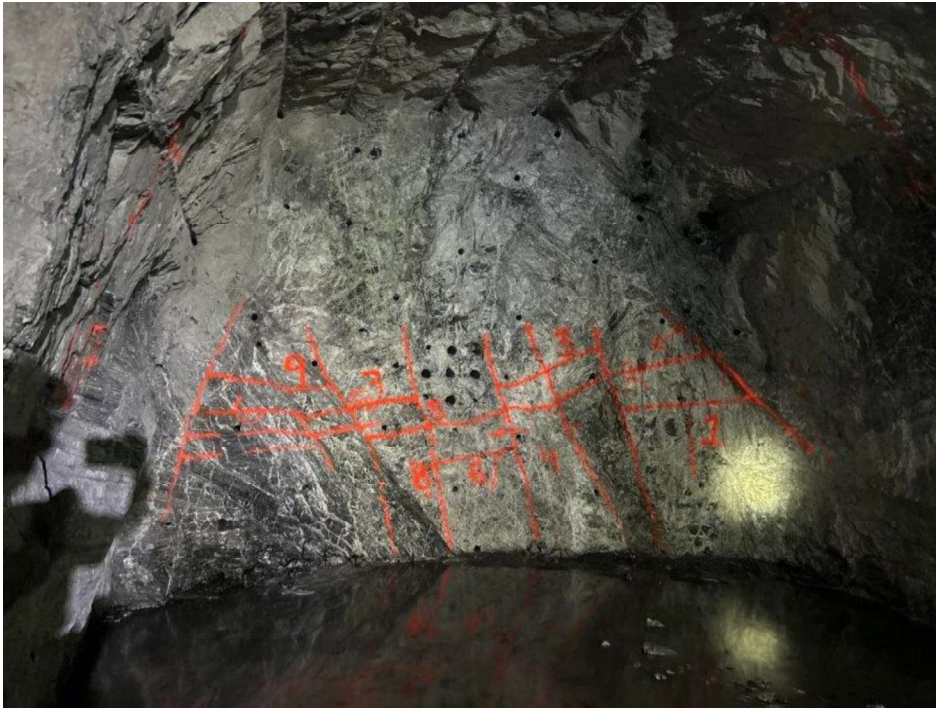
Figure 7-2: Chip-Panel Rock Sampling, Face 870-75 Segovidad Mine, Level 20
