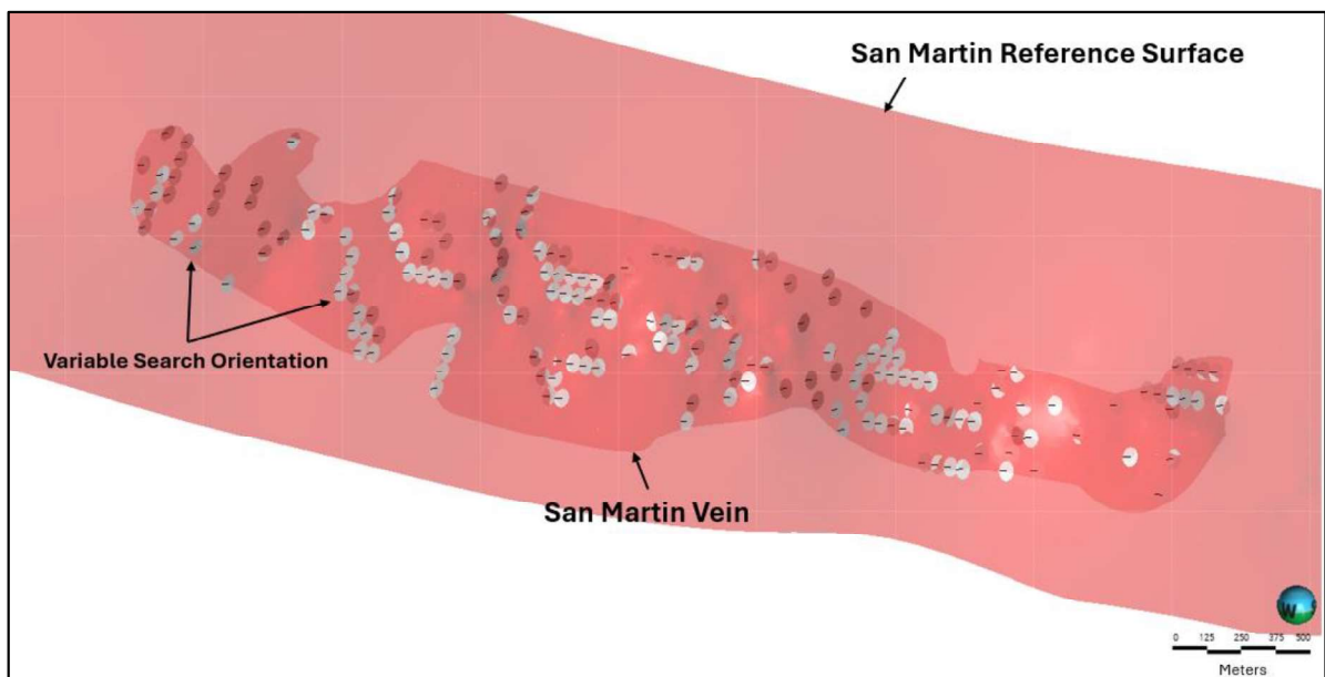
Figure 11-10: Variable Orientation for San Martin Vein
