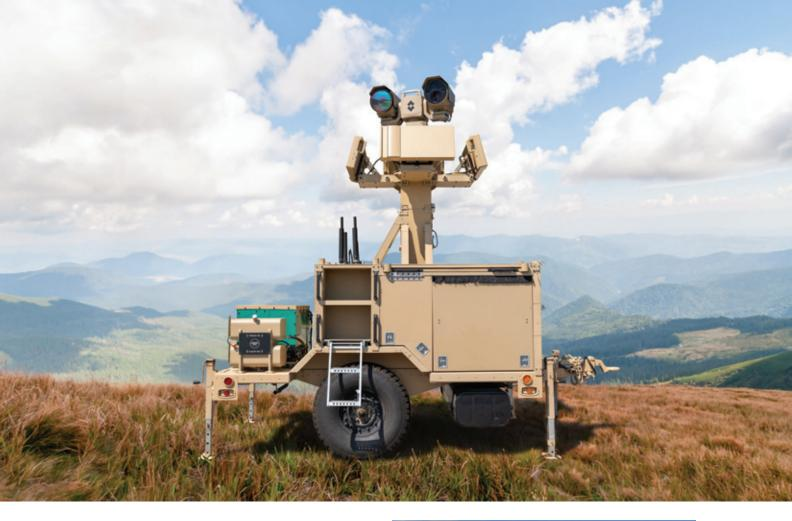
(Above and right) Teledyne FLIR's mobile counter-drone system features advanced radar, visible and infrared imaging, and is effective against drone swarms, detecting and tracking over 500 targets simultaneously.
