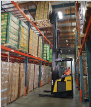
A Yale® NDR045EC narrow aisle Reach truck, designed to help enhance forward visibility when picking at height, is shown operating at a food distribution center.
