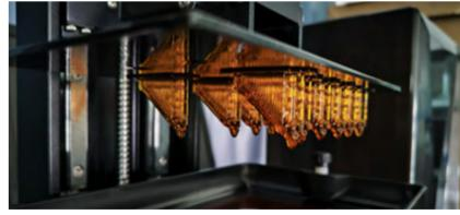
3D Printing of the Drip Irrigation Irrigator
