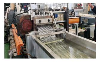
Granulating and Recycling of Scrap Material
