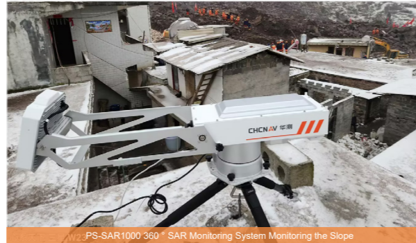
PS-SAR1000 360° SAR Monitoring System Monitoring the Slope
