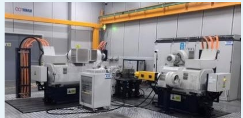
Intelligent Transmission System Comprehensive Test Platform
