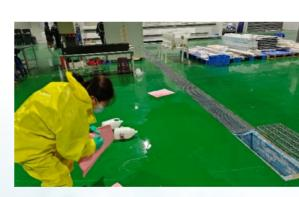
Using Absorbent Materials to Prevent Spread
