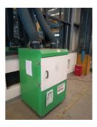
Welding fume purification with mobile dust collectors
