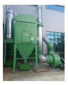
Utilizing baghouse dust collectors to achieve granularity in shot blasting lines
